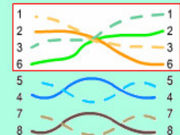
Transposed-pair Wiring Fault
