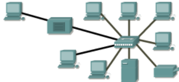
Collision Domain- Extended by Repeater
